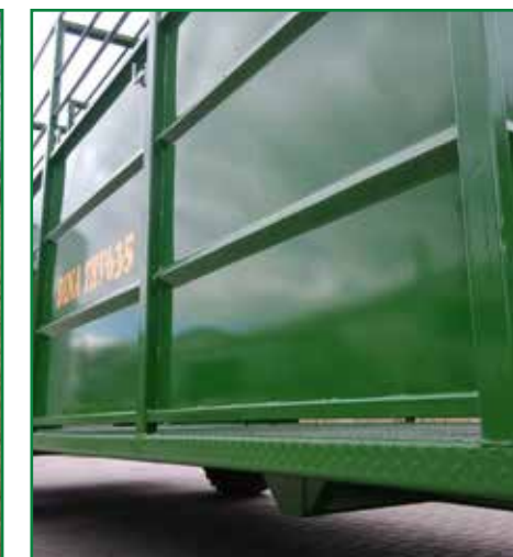
Gap around the entire perimeter for easier cleaning
