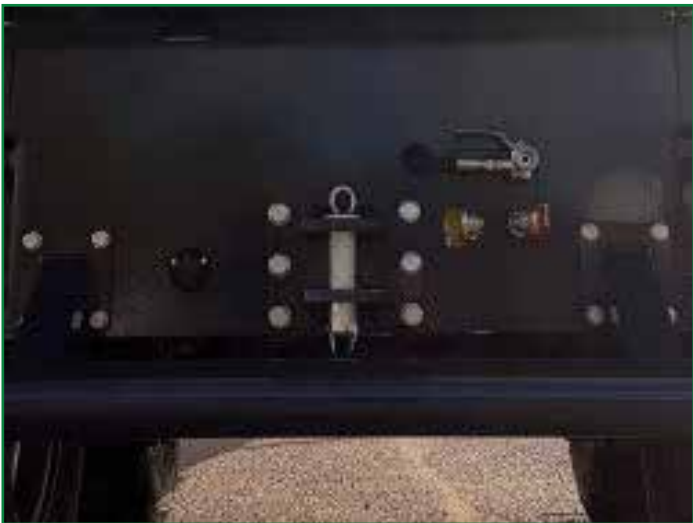
Rear towing eye with hydraulic, electric and brakes connections
